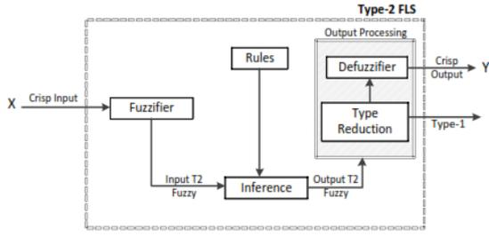
Fig 1. Type 2 Fuzzy Logic Process [15]
